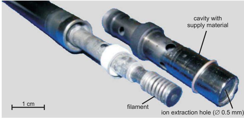
Figure 4.7: Surface ion source for alkali ions. During operation, the cavity part is mounted over the tungsten filament, which is heated with an electric power of about 30 W. The emitted electrons are accelerated by an adjustable DC voltage and heat up the ionisation surface of the cavity filled with the supply material. Ions are extracted through a 0.5 mm hole at the front plate.
